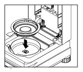
Press the **Enter** button to initiate the temperature calibration process. Follow the screen prompts throughout the process.
