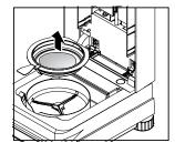
Carefully remove the sample pan handler from the drying area.
