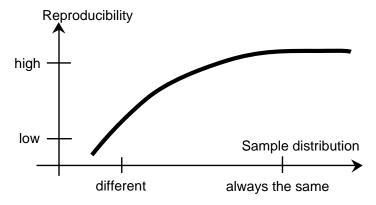
The final results of a moisture determination depends on a carefully thought out sample preparation. The part of the sample used for analysis must always be representative of the total quantity. The sample preparation includes work processes such as sampling, sample division, size reduction, homogenization and others. All of these processes should be carried out as quickly as possible and without loss or uptake of moisture.
