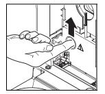
Reset the overload device with your finger. Replace the access hole cover and reconnect unit to power supply.
