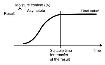
In the second type, drying runs quickly at the start and then flattens out. The moisture content never assumes a constant value. The causes of such a drying profile can be as follows:
