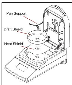
Lift the cover straight up and Install the heat shield in the base of the heating chamber.
