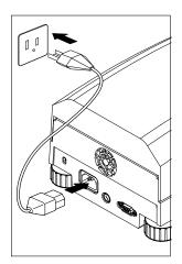
Connect the power cord supplied to the three pin connector located at the rear of the Moisture Analyzer and to a power source. The Moisture Analyzer becomes operational as soon as power is applied. The display will remain off until the **On/Off** button is pressed.
