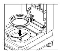
Place the empty sample pan in the pan handler (this is possible without tilting the sample pan if you insert this in the pan handler from the side directly below the round flange). Place the pan handler in the sample chamber. Ensure that the tongue of the pan handler fits exactly in the slot of the draft shield element. The sample pan must lie flat in the pan handler.
