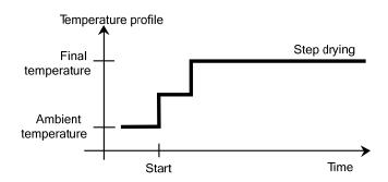
An alternate application possibility lies in the selective determination of the moisture at different temperatures. Gypsum, for example, releases only its surface water at 50°C, whereas the water of crystallization can not be separated until 168°C. With this drying program, it is thus possible to determine the surface water and the water of crystallization separately within the same measurement by a controlled temperature profile.
