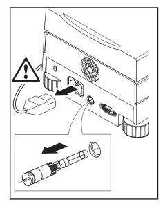
Using a screwdriver, turn the fuse holder to the left (counterclockwise) and remove the fuse.
