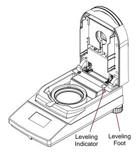
Adjust the leveling feet at the rear of the Moisture Analyzer until the air bubble in the indicator is centered. The level indicator is located under the cover towards the rear of the Moisture Analyzer.
