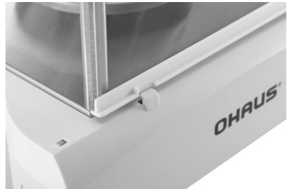
1) Install Side Doors - Insert fully into Top Frame then down over retainer.
