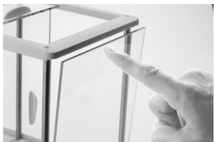
1) Install Side Doors - Insert fully into Top Frame then down over retainer.
