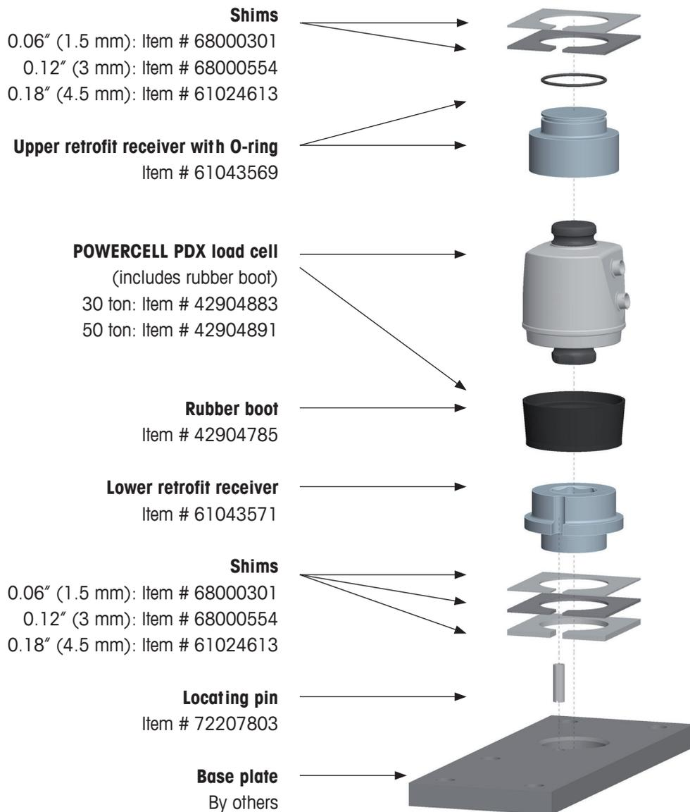
**Figure 2-4: Assembly for Receiver Variant 2 "Retrofit"**
