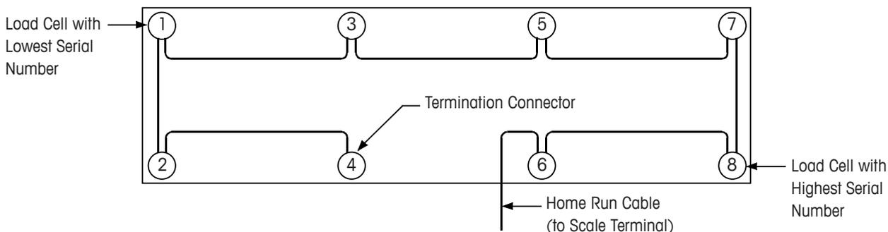
**Figure 3-5: Cable Routing for POWERCELL PDX Load Cell Network**
