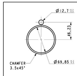
Figure 2-5: Dimensions for Receiver Variant 2 "Retrofit"
