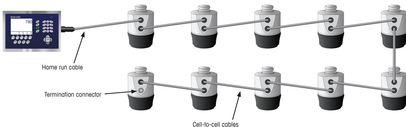
**Figure 2-6: POWERCELL PDX Load Cell Network**
