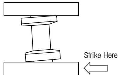
**Figure 3-4: Adjusting the Locating Tool**
