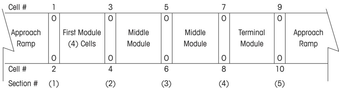
Figure 3-9: Recommended Load Cell Numbering
