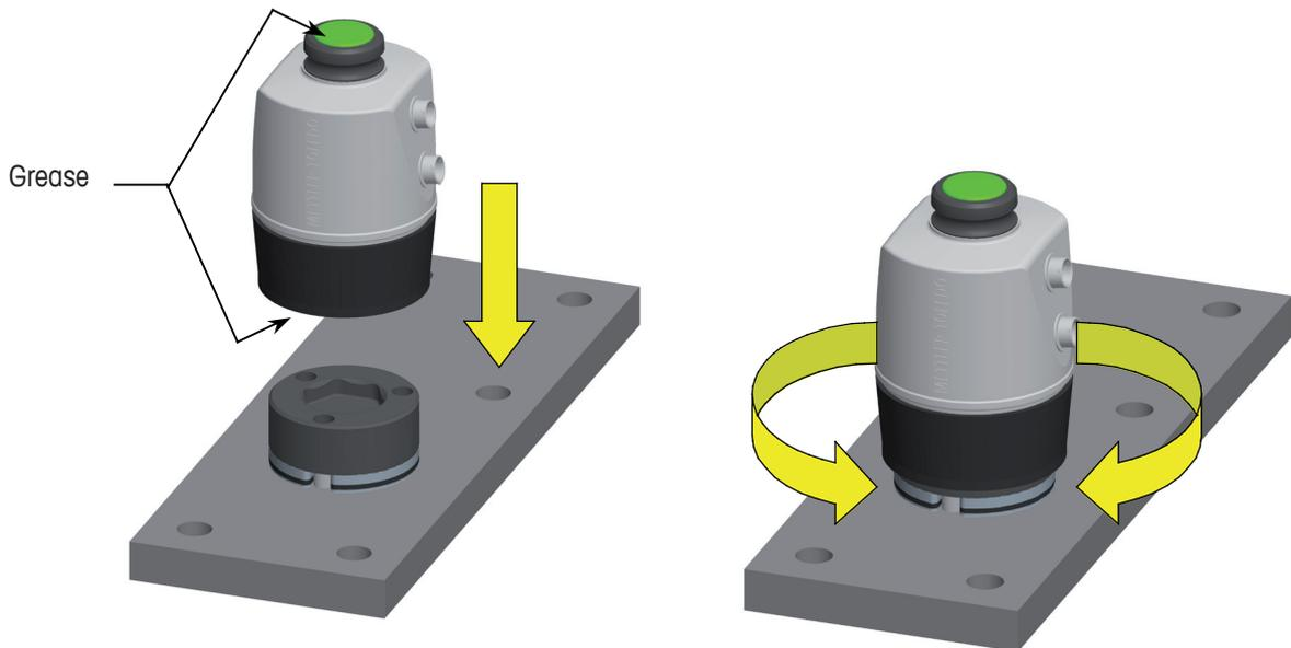
**Figure 3-6: Installing the Load Cell**
