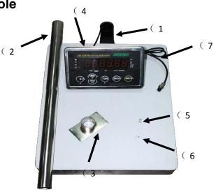
Step 1: Thread the wire of the Load Cell (9) on the rod seat (1) through the upright pole (2). Insert The upright pole into the rod seat and then lock it with two screws (5).
