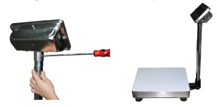
Note: Use the knob pole (7) to adjust the inclination angle of indicator and the screw (6) to adjust direction of the indicator. After adjusting the indicator to an optimal position, lock the screw.
