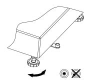
Weighing scales should be leveled precisely horizontally to provide accurate weighing results.
