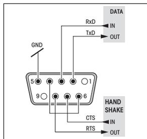
Every balance can be equipped with an optional RS232C interface for connection to a peripheral device (e.g. printer, auxiliary display or PC with a 9-pin male connector, see Section 6.4). The balance must then be configured to suit the peripheral device in a menu dialog (Sections 4.3.8 – 4.3.13).
