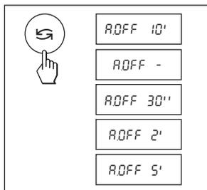
A.OFF 10' Automatic shutoff after 10 minutes inactivity
