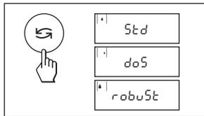
This setting allows you to adapt the balance to the weighing mode. Select "Std" (standard) for all normal weighing processes. With "doS" (dosing) - for dispensing substances in liquid or powder form - the balance reacts very rapidly to the slightest changes of weight. With "robuSt" (absolute weighing) the balance only reacts to more significant changes in weight, so that the weighing result is very stable.
