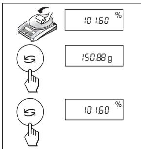
**Switching between percent weighing and weight display**
