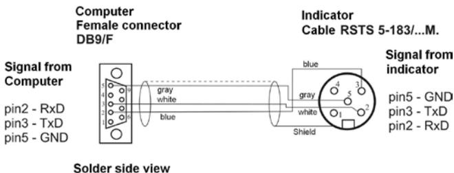
Scale – computer cable diagram for metal housing
