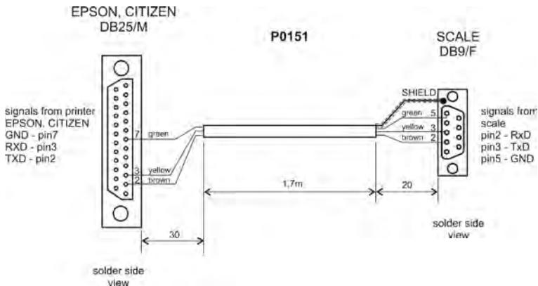
Scale – printer cable diagram for plastic casing
