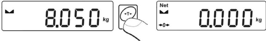
After placing a load on the weight pan net mass will be shown.
