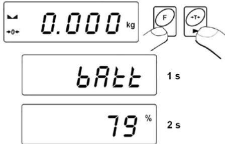
After displaying the level of batteries (in per cents) the program returns to weighing.
