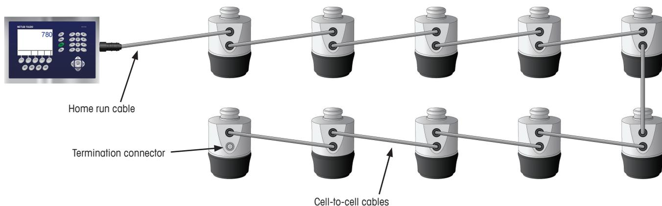
**Figure 2-6: POWERCELL PDX Load Cell Network**
