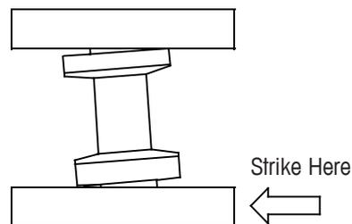
**Figure 3-4: Adjusting the Locating Tool**
